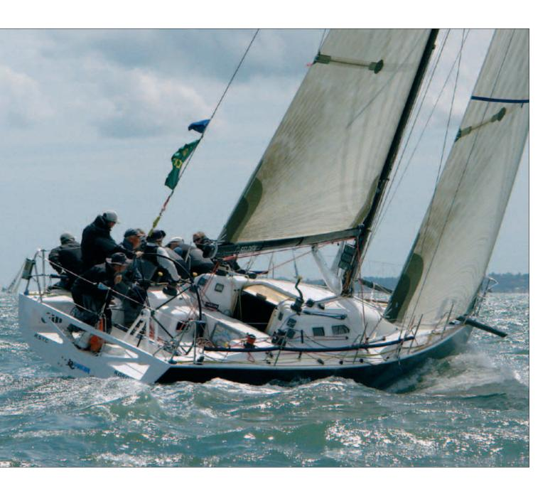
Seldén supply carbon booms that harmonise with its carbon mast range. Carbon booms offer weight savings of up to 35% compared to aluminium. This means that boom weight on a typical 35 ft boat is reduced from 30 kg to just 20 kg.
