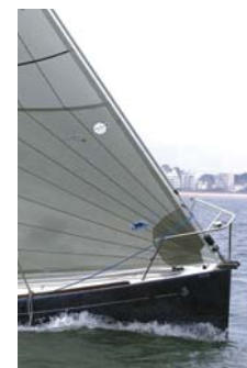
Once the half plates are removed, a racing Genoa can be hoisted using the twin groove head foil
