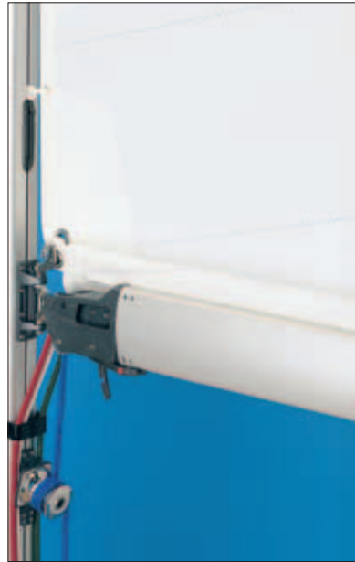
Slab reefing with fixed hooks.
