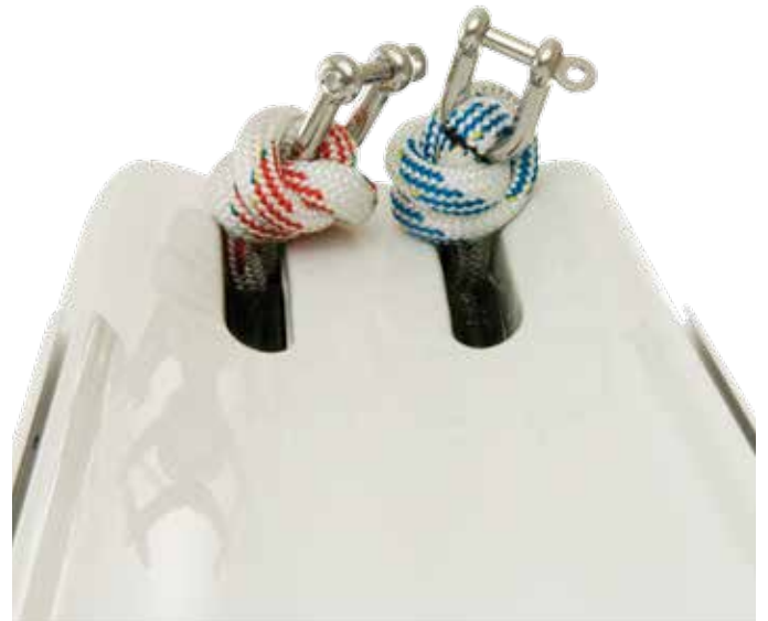
Close detailing of the concealed inboard end sheaves.
